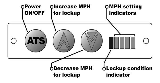
The ATS Co-Pilot will need to be set up for your vehicle and application. The Co-Pilot will need to be disassembled to access the dip switches on the electronic board. You will need a  $1/16^{th}$  - inch hex (Allen wrench) to remove the face from the Co-Pilot. After the face has been removed the
